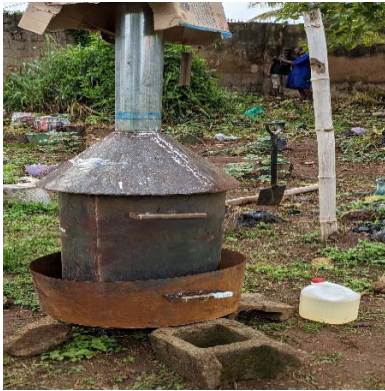
Fig1: Fabricated pyrolysis chamber
